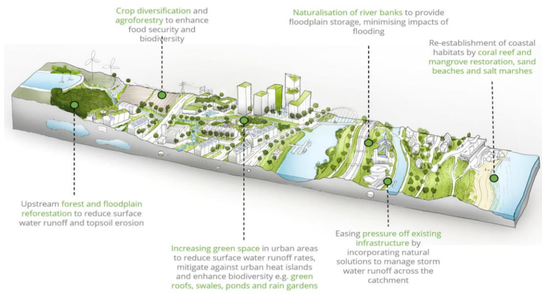
Figure 3: Watershed scale interactions and benefits of an ecosystem approach. Source: Infrastructure Pathways 5
